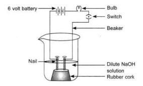
Which of the following statement(s) is (are) correct? Bulb will not glow because electrolyte is not acidic.
